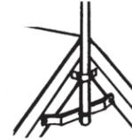
**CORNER MOUNTS:** Two Y-mounts with straps for chimney corner mounting.
