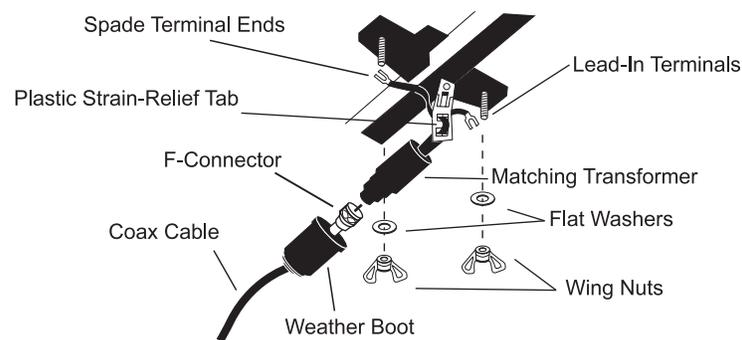
1. Split the twin-lead cable for a length of about 3 inches. Then strip about 1/2 inch of insulation from both leads.
