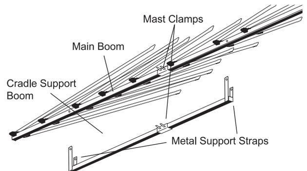
4. Press the supplied large end plugs into the main boom and cradle boom.
