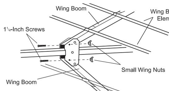
3. Fold out the wing booms and secure them into position with the two supplied 1/4-inch screws and wing nuts.
